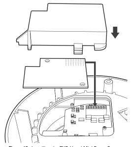
Figure 15. Installing the TXB-V and Mini Dome Cover
